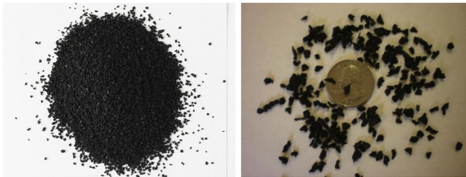
Fig. 2. Type of crumb rubber employed in this study.
