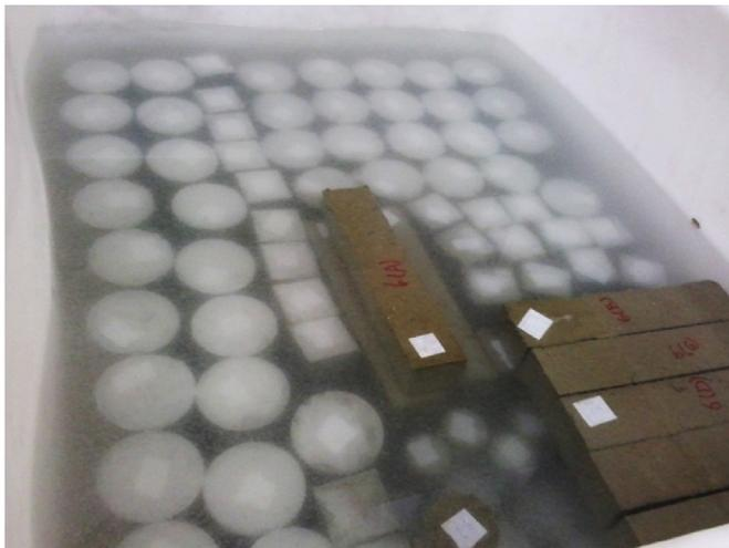
Fig. 3. Curing of specimens.
