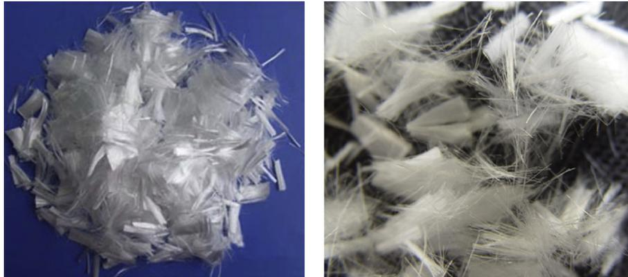
Fig. 1. Type of polypropylene employed in this study.
